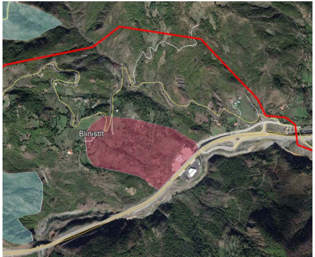
Figure 4-7: Landslide extent and pipeline route near Blinisht
