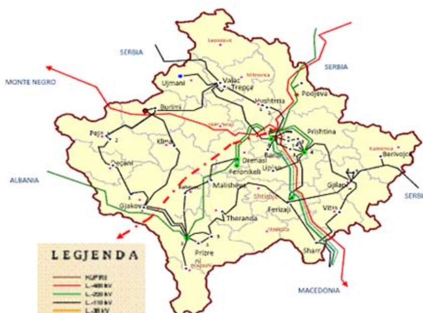
Figure 3: Interconnection of Kosovo's electricity transmission system with neighboring systems
